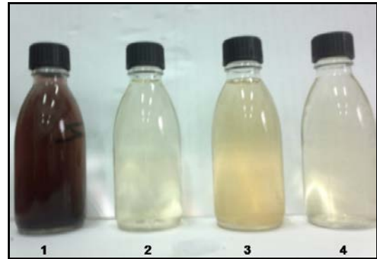
Figure 1: Real and treated wastewater samples using different electro-processes (1) real wastewater (2) treated sample using iron electrode (3) treated sample using aluminum electrode (4) treated sample using electrocoagulation/Fenton method.
